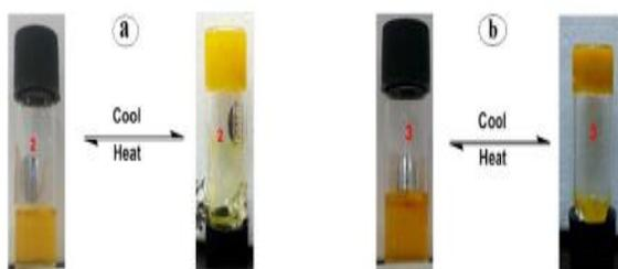
Figure 6. The thermo-reversible sol-gel transitions of the gels of ligand and complex
