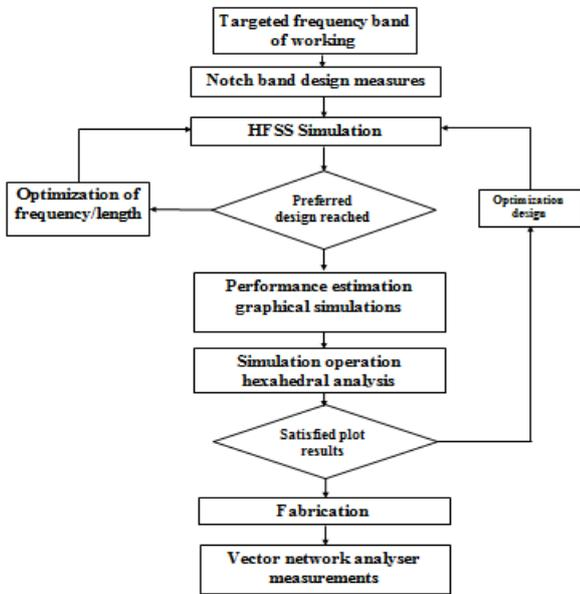
Figure 1: Operational diagram
