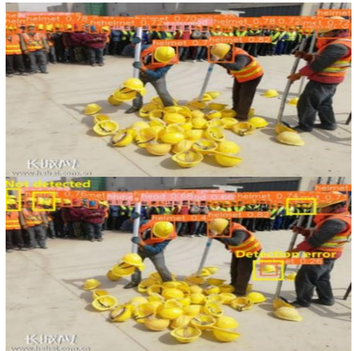
FIGURE 2. Comparison of the detection performance in various real-world application scenarios between YOLOv8n and YOLOv8n-SLIM-CA
