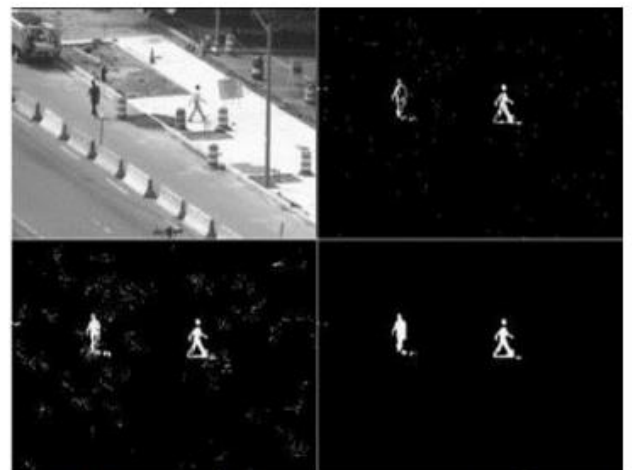
Fig. 1: Example of object detection by background removal
