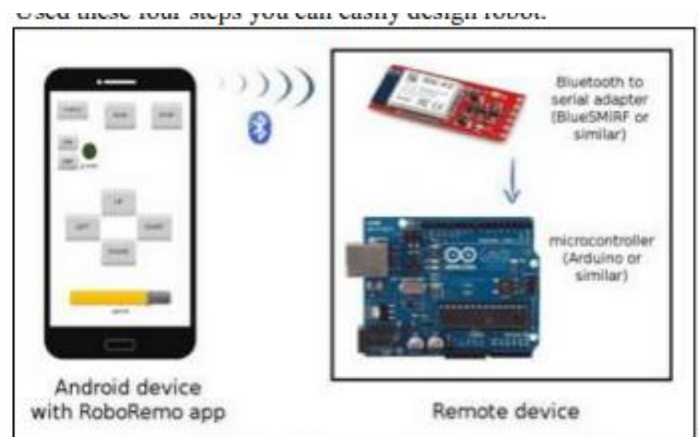
Fig. 4.3: Interfacing of Bluetooth Module & Android Phone
