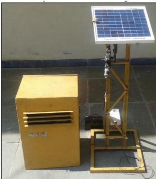
Fig. 1: Physical Setup of Solar Air Cooler with Auto Tracker
