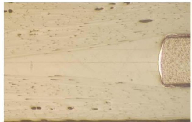
Figure 2: Micro-graph of a section of S-glass/epoxy composite laminate with embedded simulated micro sensor
